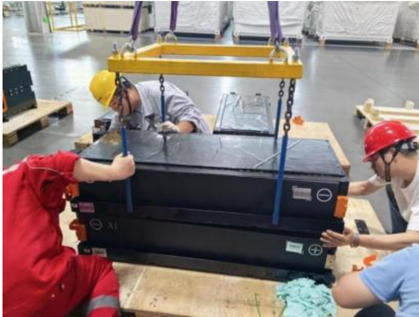
picture 9-17 Schematic diagram of battery module lifting points
