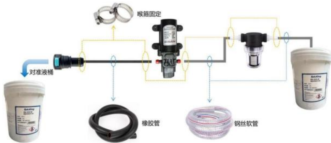
picture 9-31 Injection fixture (fixture emptied)
