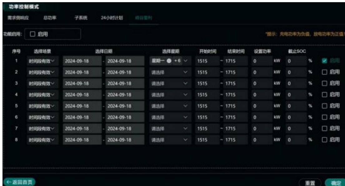
picture 7-14 Peak-Valley Arbitrage Setup
