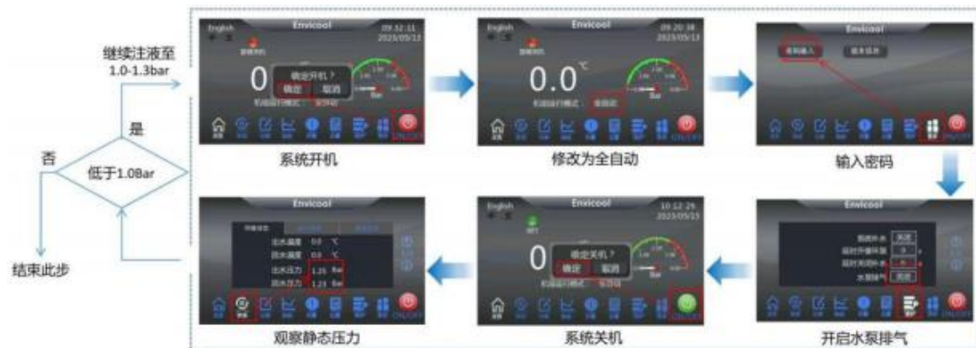
picture 9-35 Schematic diagram of commissioning and exhaust process
