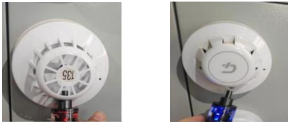
picture 9-1 Detector sensing test
