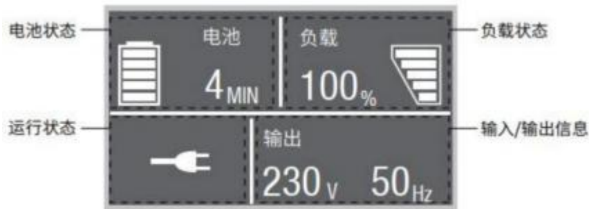
picture 9-14 UPS display screen interface
