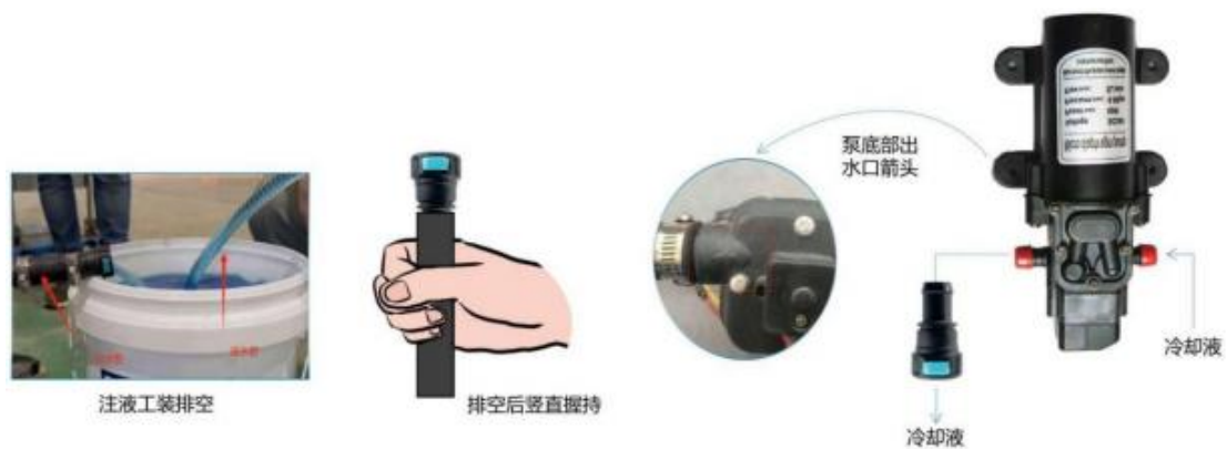
picture 9-32 Schematic diagram of the liquid injection tooling emptying process
