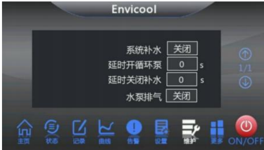
picture 9-13 Maintenance Interface
