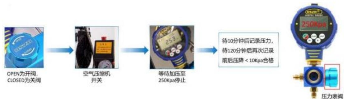
picture 9-28 Pressure holding process diagram
